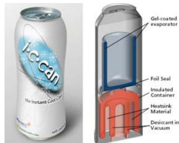
Gambar 4.36. Self cooling packaging
